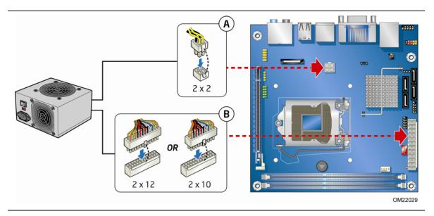
Figure 23. Connecting Power Supply Cables
